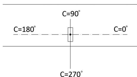
Figure 4.12 Orientation of C half-planes in case of road lighting luminaires
