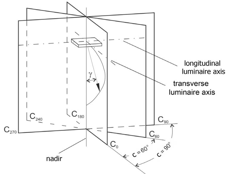
Figure 4.10 Standard C- $\gamma$  system for recording the luminaire luminous intensity table
