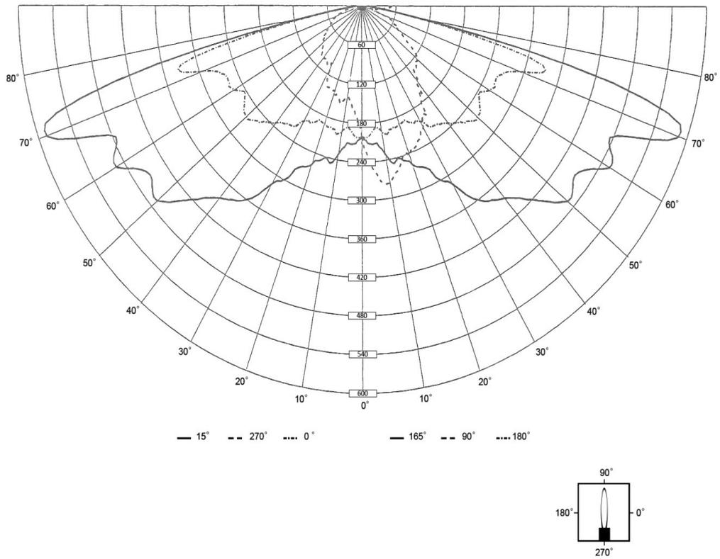
Figure 4.13 Polar diagram of a road lighting luminaire
